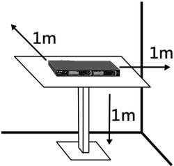
For best operation, the receiver should be at least 1m above the ground and 1m away from a wall or metal surface to minimize reflections. The transmitter should also be at least 1m away from a wall or metal surface to minimize reflections. The transmitter should also be at least 1m away from the receiver. Keep antennas away from noise source such as motors, automobiles, neon light as well as large metal objects.
