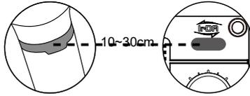
Align infrared areas of the receiver and microphone within 10~30cm.
